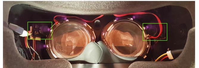
Figure 8. Additional HMCs are attached next the Fresnel lenses (green boxes). We crafted two printed circuit boards (PCBs) with 9 IR LEDs each. They cover the original IR LEDs for eye tracking of the HTC Vive Pro Eye which are located around the Fresnel lenses. This was done to avoid image artifacts in the streams of our HMC for eyebrow tracking.
